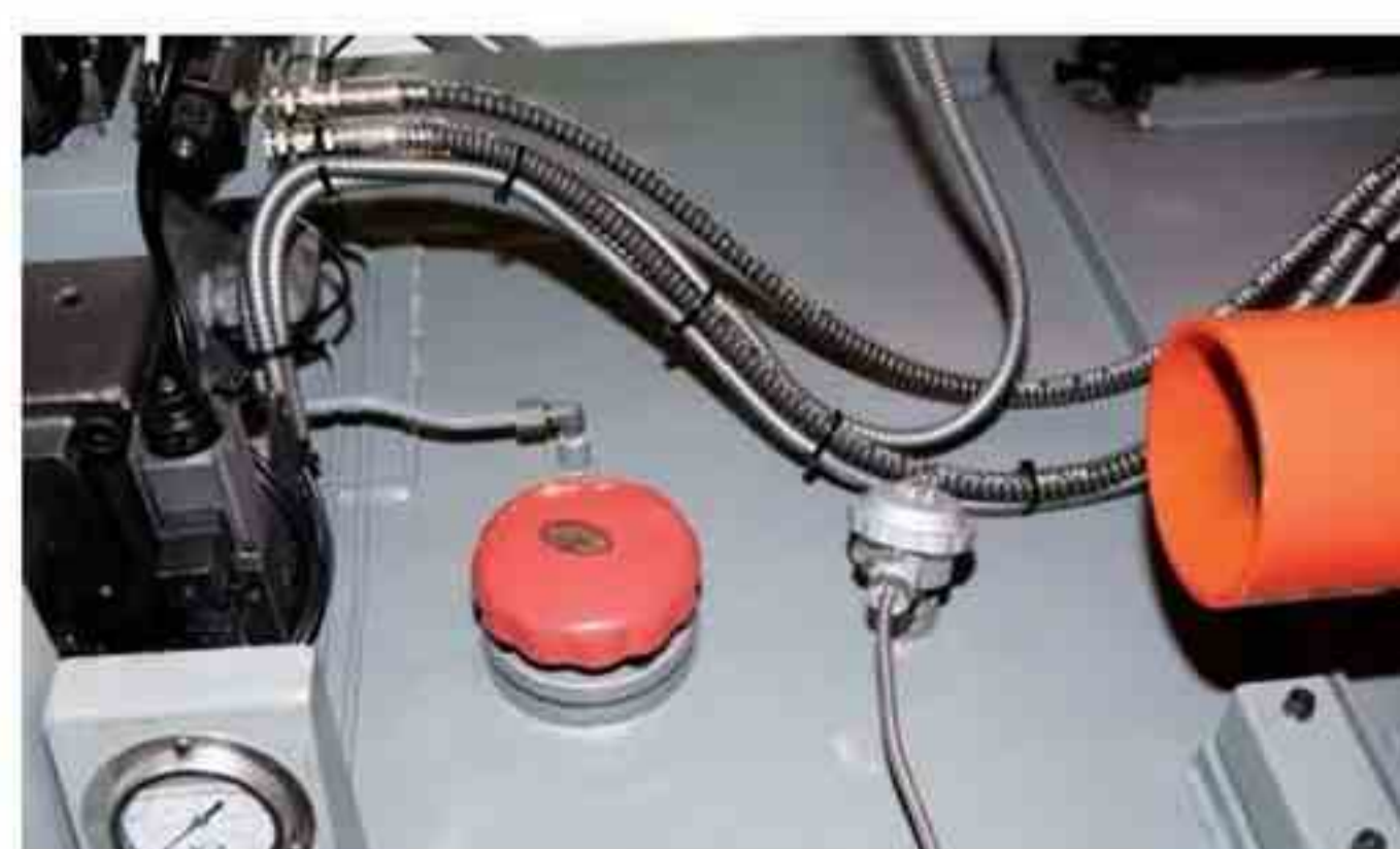
特有的油温探测仪 Special oil temperature sensor
