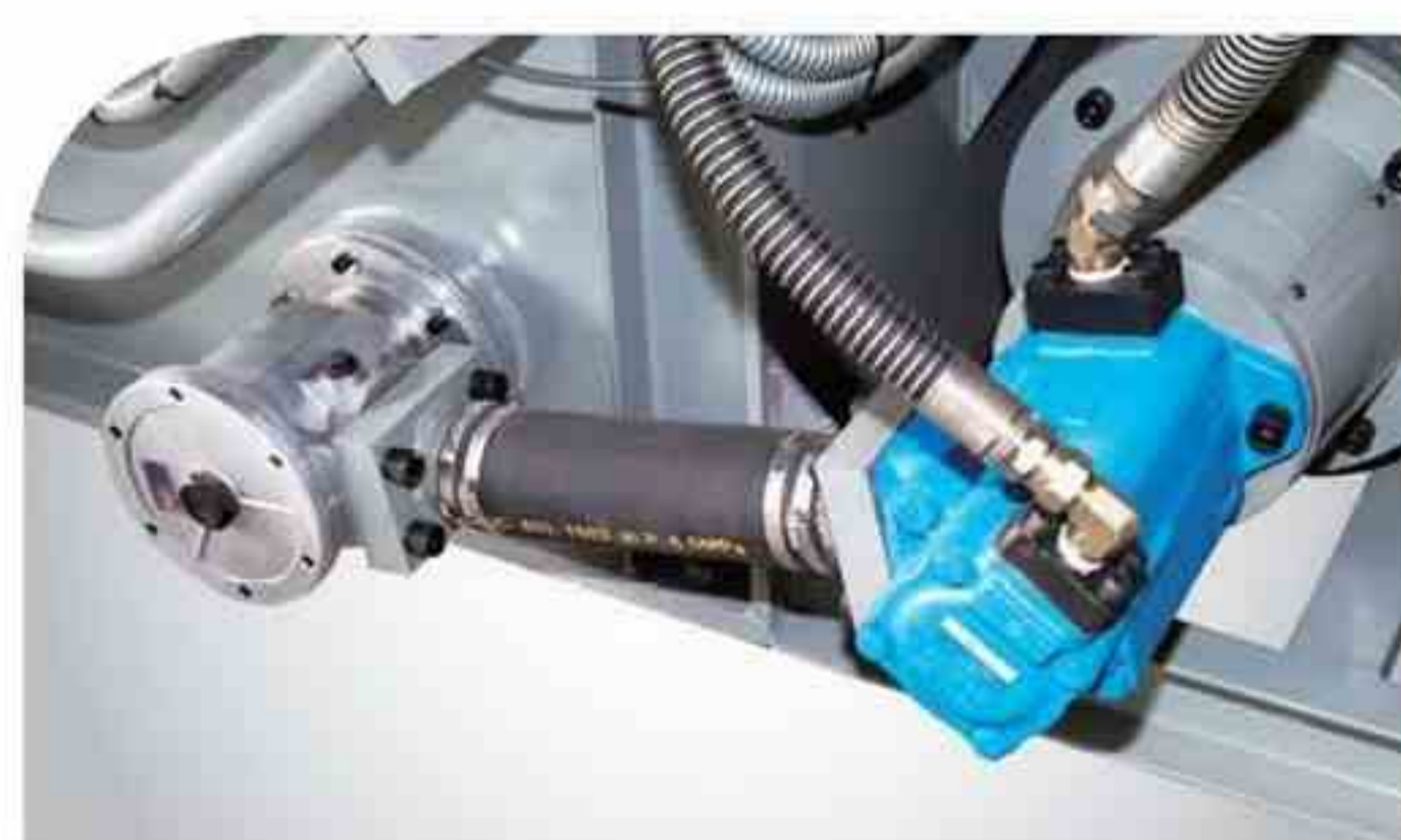
进口名牌高性能高低压双联泵 Imported high quality dual-pump
