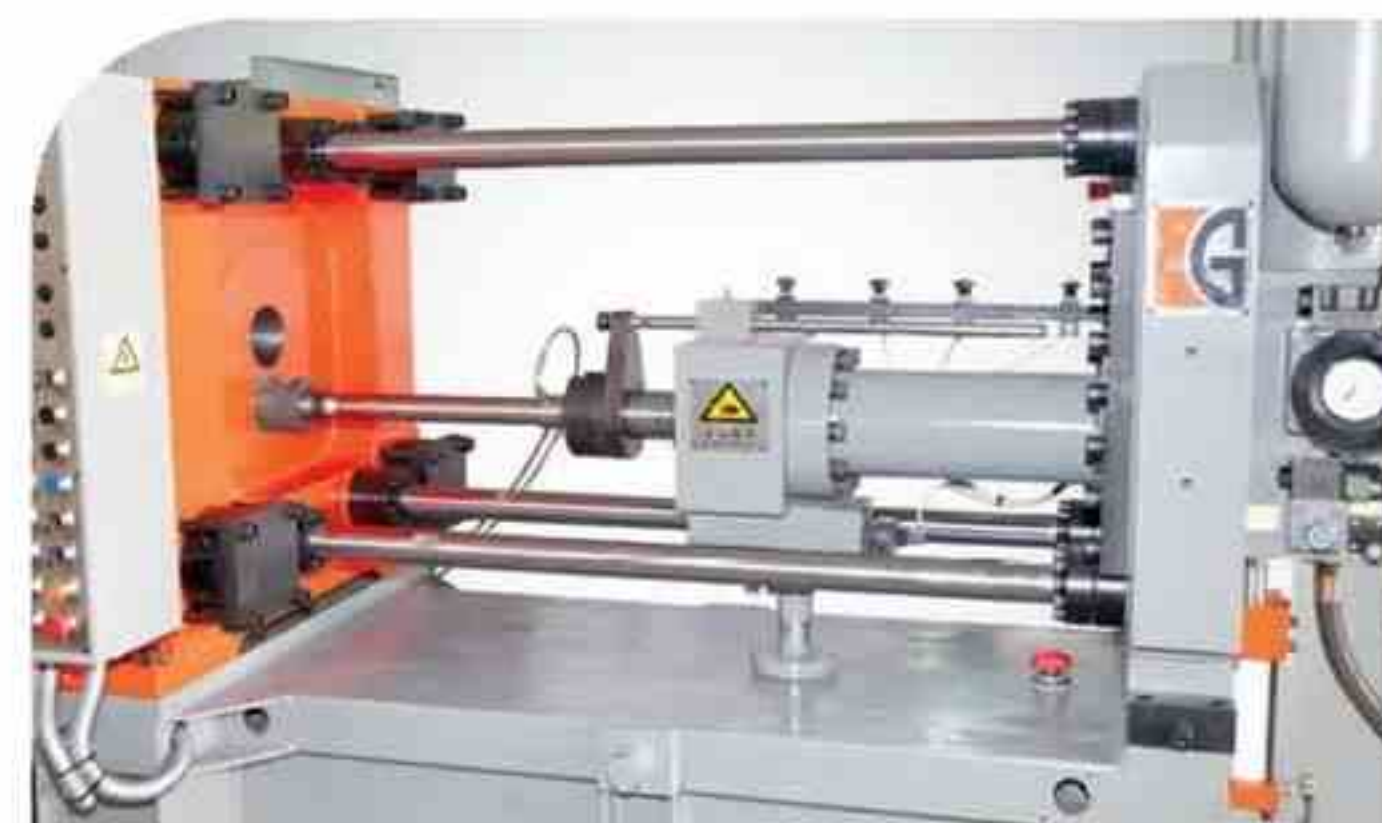
四拉杆式结构、三级压射的调整控制 Rod type structure , three stage injection adjustment
