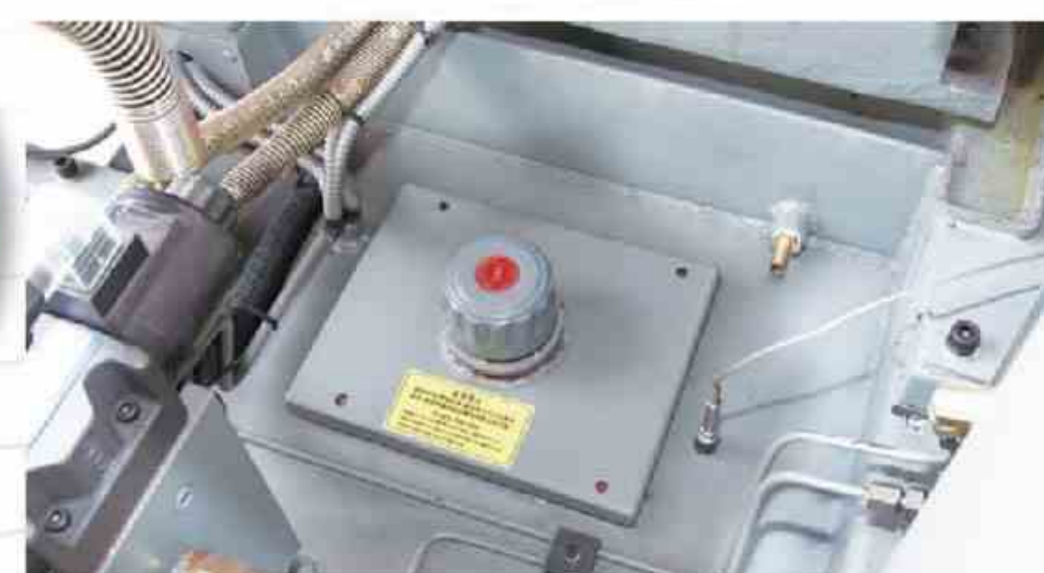
特有的油温探测仪 Special oil temperature sensor
